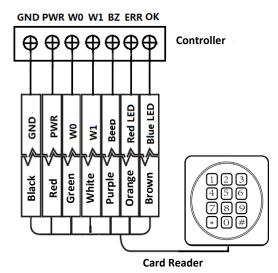
**Note:** You must connect the OK/ERR/BZ, if using access controller to control the LED and buzzer of the Wiegand card reader.
